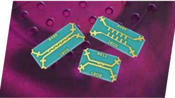
DLI's surface mount directional coupler series span the frequency spectrum of C, X and Ku bands. Both 10dB and 20dB coupling values are available within each frequency band both with a common footprint for maximum flexibility. These couplers incorporate DLI's low loss high permittivity ceramics which provide small size and temperature stability. These couplers offer a turnkey surface mount solution for high frequency power monitoring. Custom solutions are also available.
