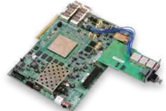
FMC+ HSPC Loopback Card Supporting Xilinx® Virtex® UltraScale™+ VCU118 Kit
