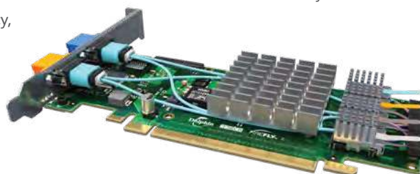
PCI Express®-Over-Fiber Adaptor Card
