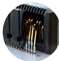
Differential pair for increased speed (HSEC8-DP)
